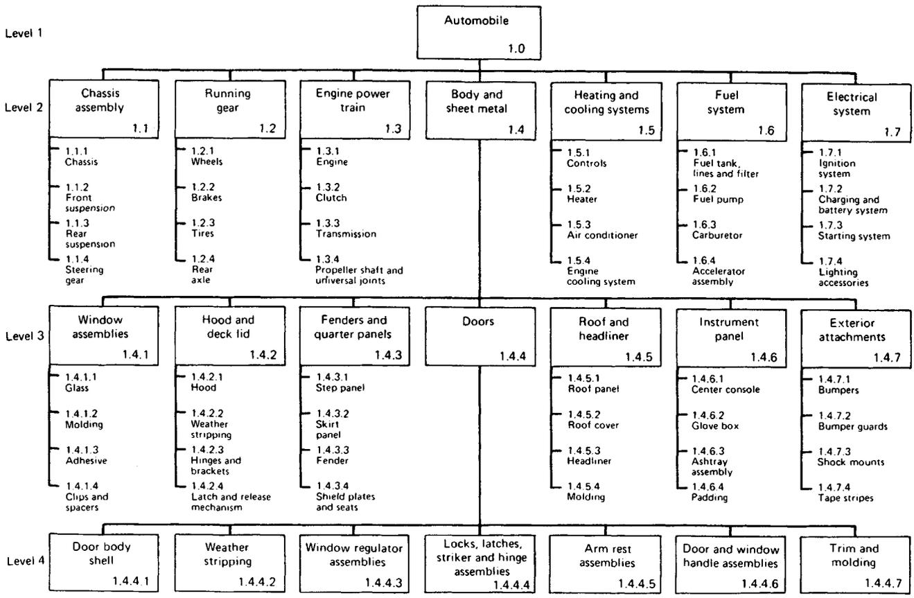
Fig. 70.4 Work breakdown structure of an automobile.
